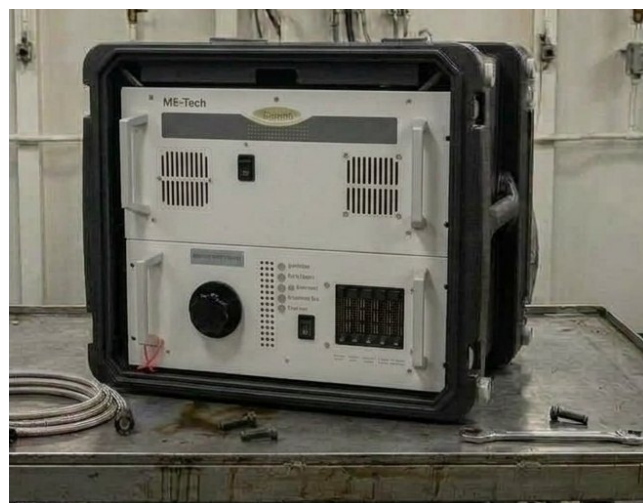
FTIR analyzer onboard, used for N 2 O, methanol and formaldehyde.
